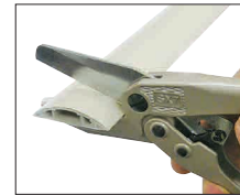
Cutting of cable protector
