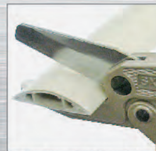
Cutting of cable protector
